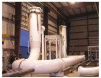
the piping system. Flanges in the pre-run are aligned using shoulder bolts that are approximately the same diameter as the flange bolt holes. Not having to cut or drill a flange is a safety improvement.
